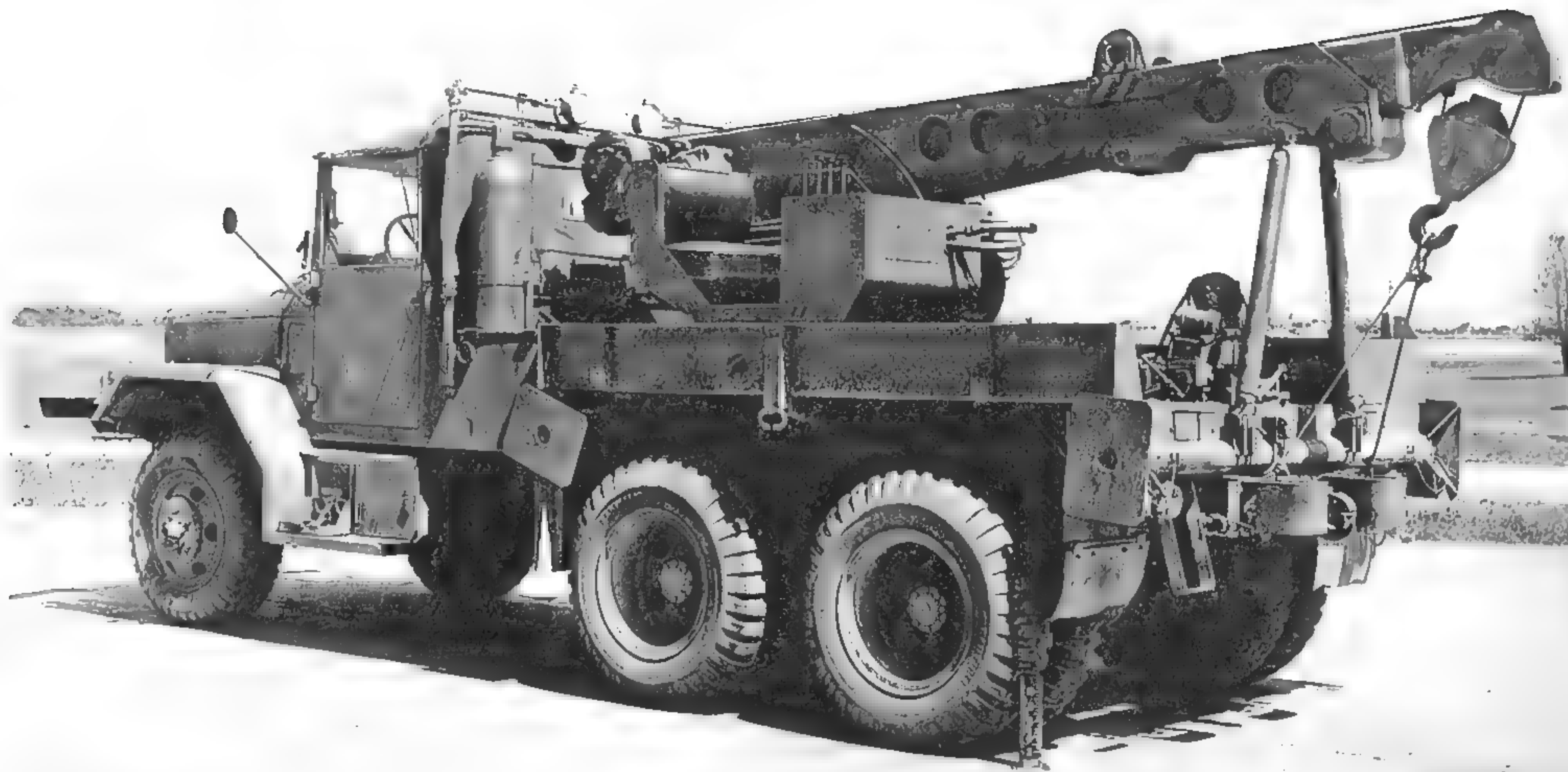
The XM60 bed had sideboards to retain the recovery equipment it carried, and a large winch was mounted in the rear of the bed. (Photo courtesy of the Patton Museum)
